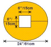
Column Sentry® CS2442-8x10H column protector is designed to fit around columns with an 8"(20cm) web and flanges up to 10"(25cm). The outside diameter is 24" (61cm) \*NOTE: PLEASE MAKE SURE THE WEB IS 8"! WILL NOT FIT 10" WEB.
