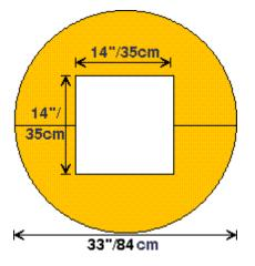
Column Sentry® CS3342-16S column protector is designed to fit around H, square, or round columns up to 16"x16"(40x40cm) in diameter. The outside diameter is 33" (84cm)
