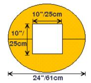
Column Sentry® CS2442-12S column protector is designed to fit around H, square, or round columns up to 12"x12"(30x30cm) in diameter. The outside diameter is 24" (61cm). Available in either standard or FE type for Fire Extinguishers
