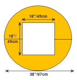
Column Sentry® CS3842-20S column protector is designed to fit around H, square, or round columns up to 20"x20" (51x51cm) in diameter. The outside diameter is 38" (97cm)
