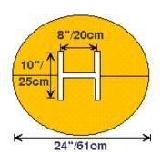
Column Sentry® CS2442-8S column protector is designed to fit around H, square, or round columns up to 8"x8"(20x20cm) in diameter. The outside diameter is 24" (61cm). Available in either standard or FE type for Fire Extinguishers
