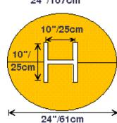
Column Sentry® CS2442-10S column protector is designed to fit around H, square, or round columns up to 10"x10"(25x25cm) in diameter. The outside diameter is 24" (61cm)
