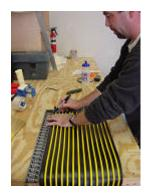
Step 2 – Measure length of Bumperwrap™ to match the circumference of the object, and cut to the determined length. A sharp utility knife or heavy-duty scissors will work well for cutting Bumperwrap™. For best results, use a metal framing square or similar tool to ensure a square cut. Check the length by wrapping the cut piece tight around the object, leaving ½" gap for the fasteners. When wrapping the same size object in several applications, complete first installation to check for a good fit.
